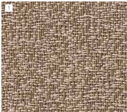
1. PU-coated woven wear side
